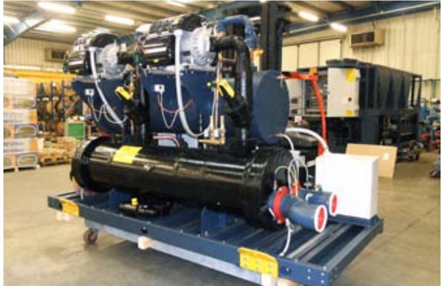
finished product are paramount. Turbomiser provides a steady supply of chilled water or glycol at design temperatures +/- 0.5 °C to cool the food and beverage process equipment. Turbomiser has the advantage that it does not require potentially expensive oil and filter changes and there are no oil pumps or heaters to worry about. It's clean technology perfectly designed for the food and drinks industry.
